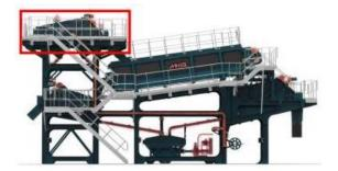
The Pre Screen is a primary rinsing screen before material enters the Logwasher hull. Material going to this screen will have passed through a tipping grid, or a scalping screen to size at 100mm (-4") On this screen the material will be rinsed to remove the majority of -5mm material. Reducing the amount of 5mm in the log washer hull is imperative to increase the function of stone on stone attrition for scrubbing the material & also reducing wear on the blades
