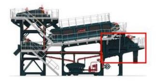
After passing through the Logwasher Hull, the cleaned Aggregate is transferred onto a second screen. There are a number of different options for this screen. The single deck screens are used for rinsing the material before transferring onto a secondary sizing screen. The incline screens are used for sizing and rinsing directly from material discharge of the log washer hull. Further information on material flows can be found in the flow sheets later in this document
