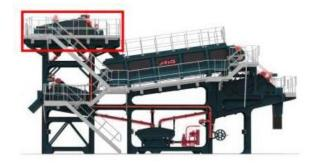
The Pre Screen is a primary rinsing screen before material enters the Logwasher hull. Material going to this screen will have passed through a tipping grid, or a scalping screen to size at 100mm (-4") On this screen the material will be rinsed to remove the majority of -5mm material. Reducing the amount of 5mm in the log washer hull is imperative to increase the function of stone on stone attrition for scrubbing the material & also reducing wear on the blades
