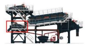
Trash Screen is located at the back end of the hull. Its purpose is to deal with any woods, plastics, or light material that weirs off the back of the logwasher, dewater the trash material and discharge into a bay or skip to improve the quality of the end product
